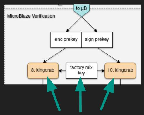
FPGA fabric secrets used to derive user keys using kingcrab FPGA module
